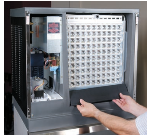
Lift cascading shield off photo-eyes, rotate forward and out of the machine.
