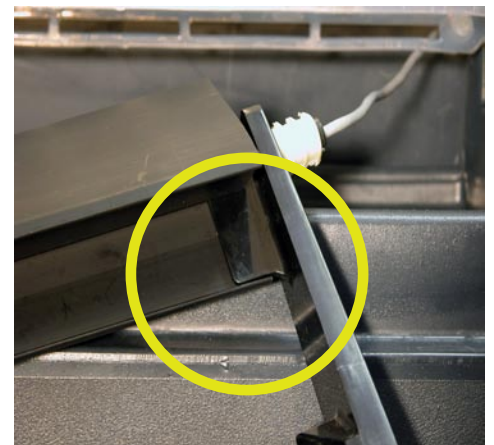
Note how cascading shield snaps onto photo-eye mounts.
