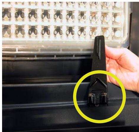
Photo eye holder out of machine. Clean photo eyes. Reverse steps to reassemble.
