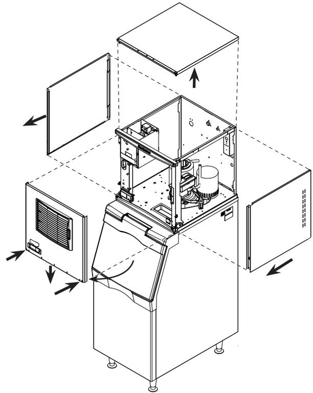
1. Locate and loosen the two screws at the bottom of the front panel.
