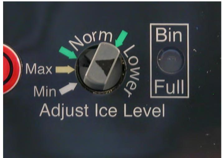
Rotate the adjustment post to the desired ice level.
