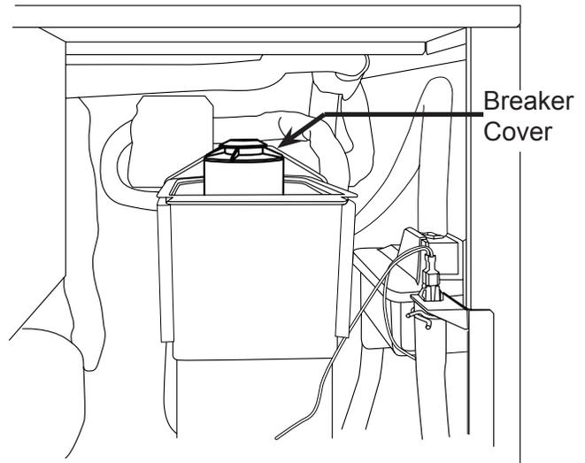
3. Removing the water shed & unscrewing the breaker cover (left hand threads).
