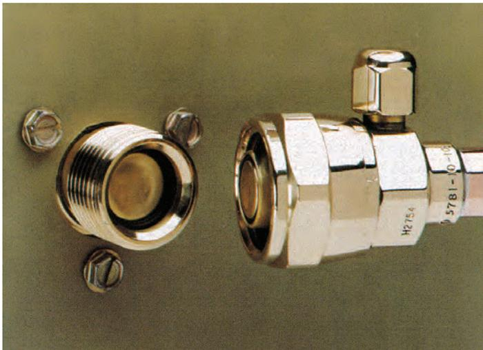
5. Use two wrenches tighten the coupling until it bottoms out or a definite increase in resistance is felt. It is important that ONLY the nut on the pre-charged tube be turned, or the diaphragms will be torn out by the piercing knives and they will be loose in the refrigeration system.
