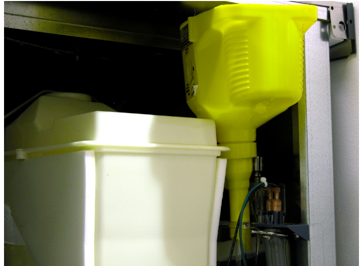
10. Insert funnel in reservoir,
