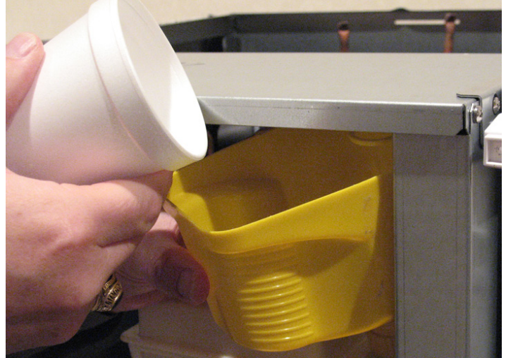
11. Add scale remover solution to reservoir.
