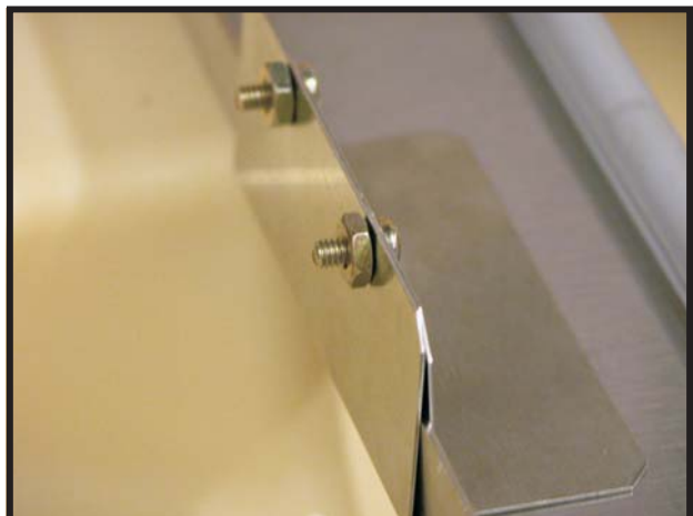
Secure Cap Tube Mounting Bracket to Adapter Flange
