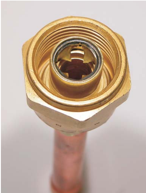
Pierced but will leak
