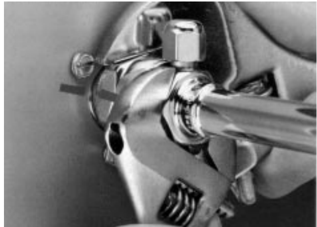
Tighten Swivel Nut
