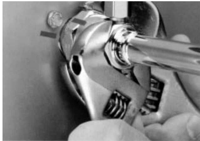
Rotate Swivel Nut ¼ Turn More
