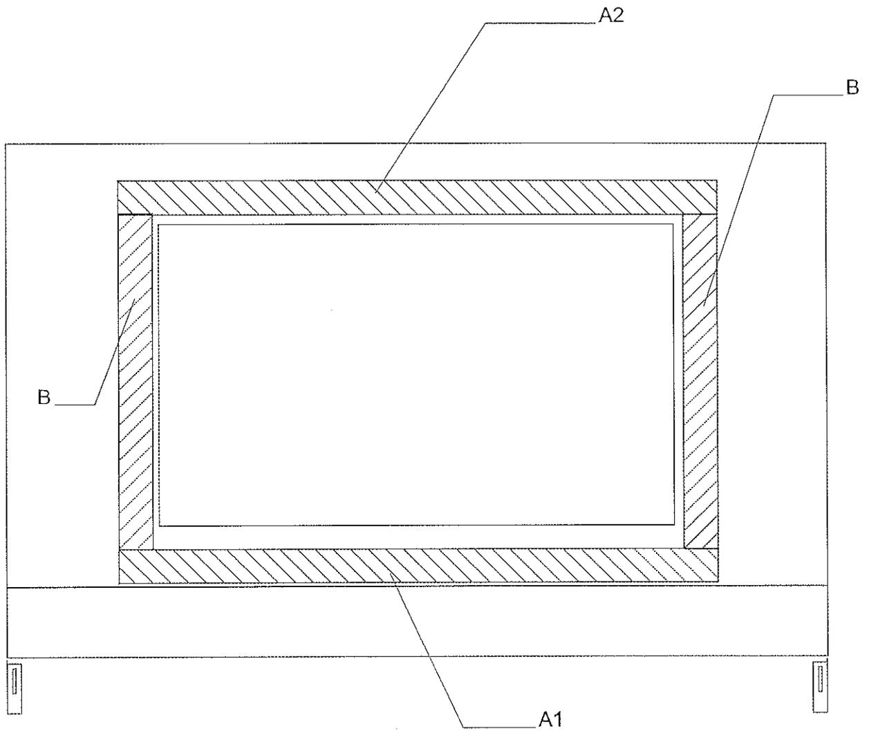
Place 22" gasket (A1) flush with front edge of top surface as shown, 4 1/8" from left & right ends.
