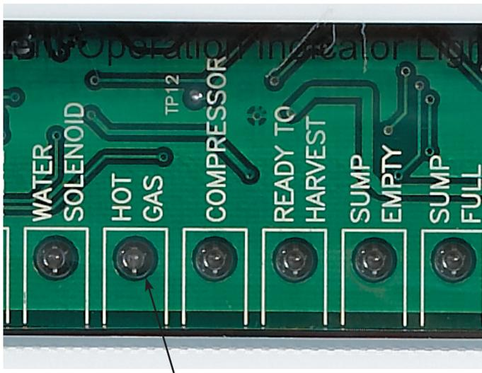
This light will be ON when the Hot Gas Valve and Harvest Assist have power.
