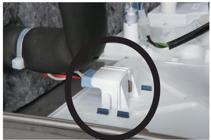
Water touching the sensor's short probe triggers the Sump Full light. No water touching the mid-length probe triggers the Sump Empty light. During most of the freeze cycle neither light will be on.
