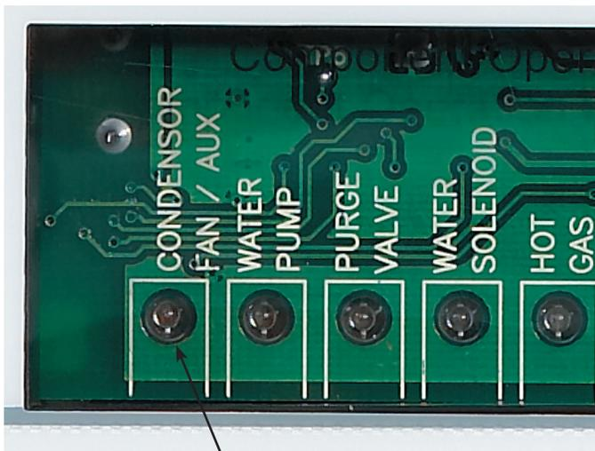
This light will be ON when the liquid line solenoid has power.
