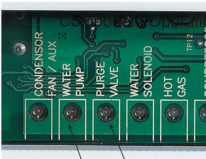
Only one water pump is ON when the purge valve light is ON
