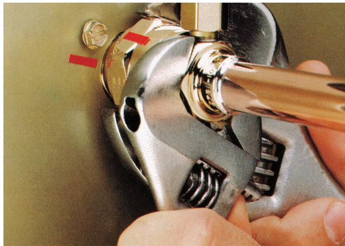
quarter turn. The line will show the amount that the nut turns. Do NOT over tighten.
