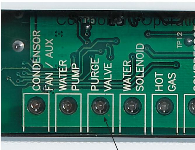
This light will be ON when the Purge Valve is ON.
