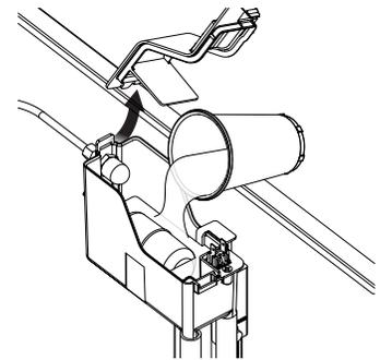
18. Drain the water from the water system by pulling the reservoir drain hose from its plug and return it to the plug when drained.
