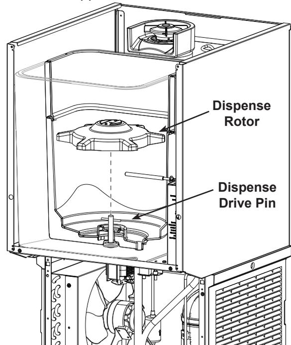
12. Use a clean cloth and wash all the interior surfaces of the bin and the bin cover, agitator bar, chute cover and dispense rotor with the ice machine scale remover solution. Rinse with clear water.
