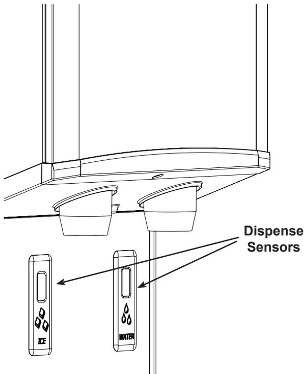
If the user does not remove the container, ice will be dispensed for 24 seconds and then stop.
