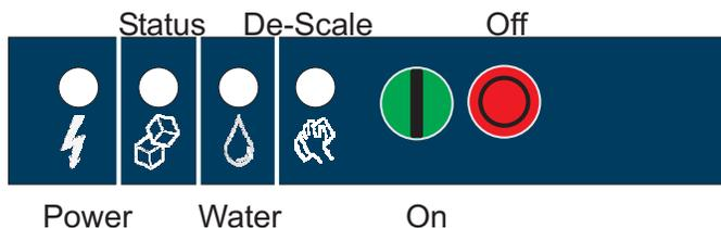
To switch the machine ON, push and release the On button. The machine will go through a start up process and then resume ice making.
