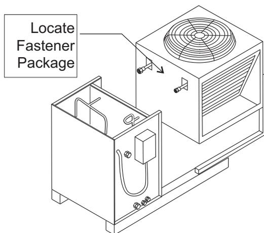
6. Assemble rear legs to ERC using fasteners from prior step.
