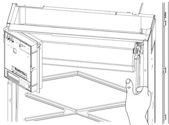
**Release Controller Mounting, Swing Forward.
