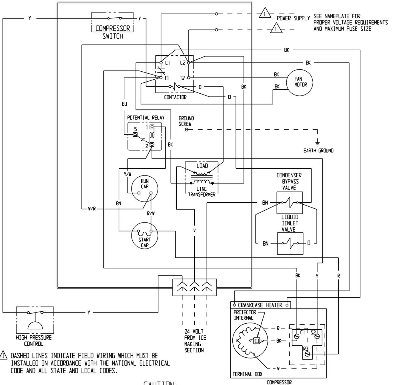
⚠ DASHED LINES INDICATE FIELD WIRING WHICH MUST BE INSTALLED IN ACCORDANCE WITH THE NATIONAL ELECTRICAL CODE AND ALL STATE AND LOCAL CODES.
