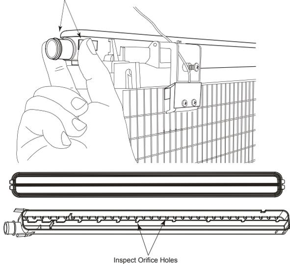
12. Locate water level sensor. Squeeze catches together and pull up to remove sensor.
