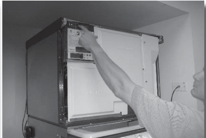
17. Re-assemble panels and Push On to start machine.
