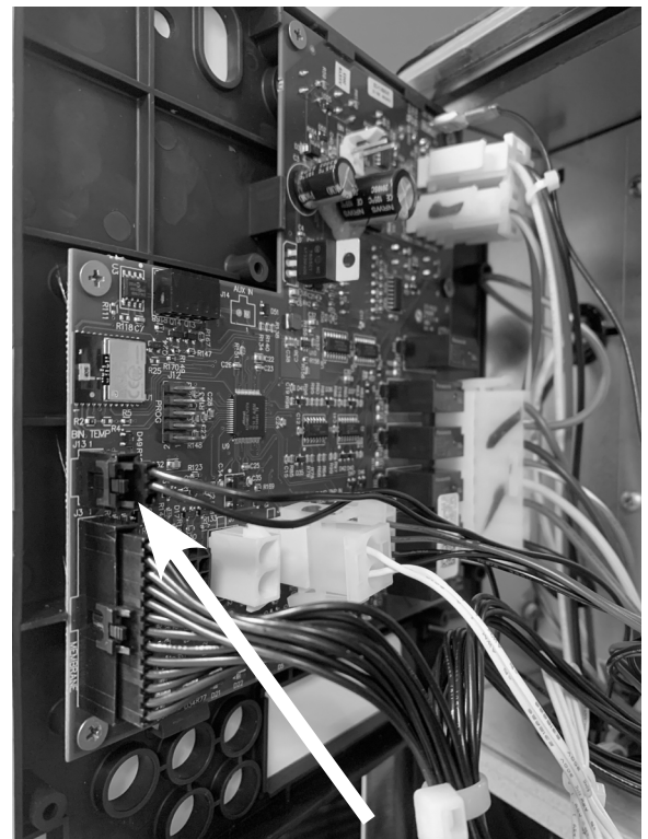
Connect to control board at J13
