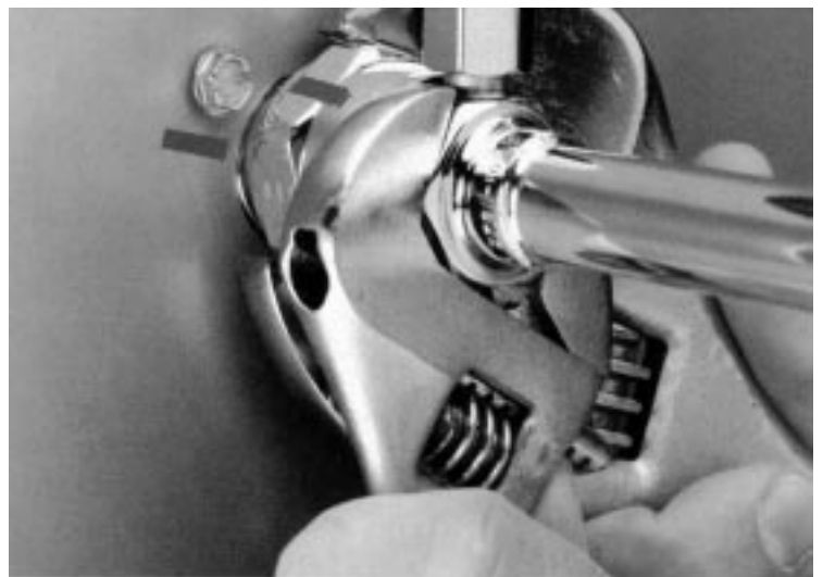
Rotate Each Swivel Nut ¼ Turn More
