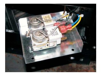
9. Disconnect wires from cube size thermostat.
