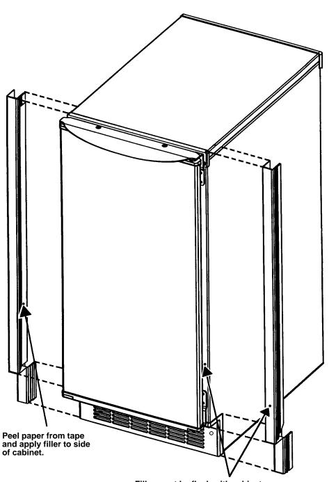
Filler must be flush with cabinet front and even with top of cabinet.
