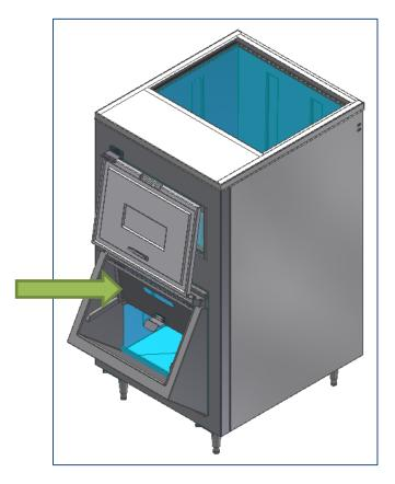
1. Locate the baffle assembly by lifting the snout door up.
