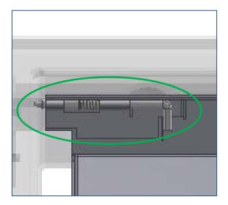
2. Looking at the baffle assembly from the front of the bin, locate the spring latches underneath the top lip.
