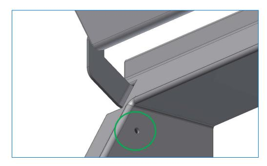
3. Locate the spring latch mounting holes inside the snout walls.
