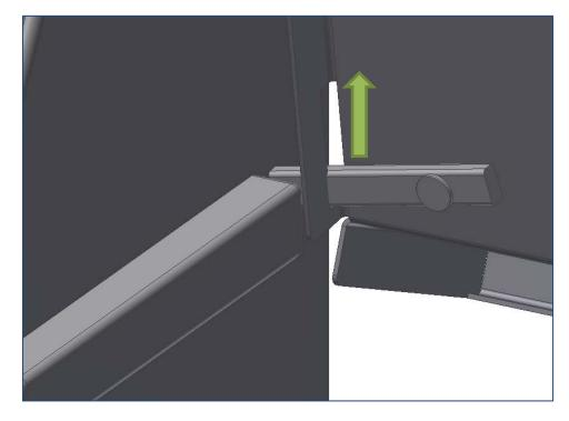
5. Once rotated forward, lift the assembly up and over the pivot arm catches.
