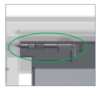
1. Locate the spring latches underneath the top lip of the baffle assembly.
