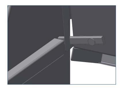
6. Slide the assembly back until it's past the pivot arm catch, then release the pivot arms to lock it in place.
