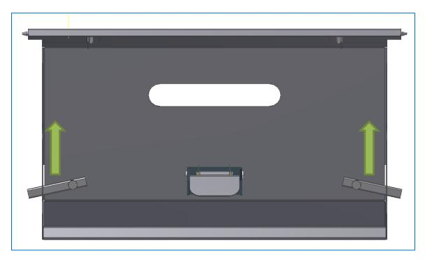
4. Locate the baffle assembly and release the spring latches into the mounting holes.
