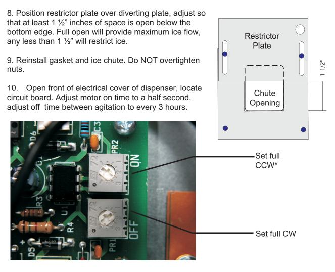
11. Reconnect power, agitator should cycle a half second\*. Check ice shutter operation.
