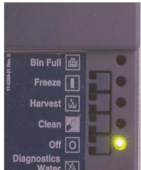
**To Test:** Move the float stick slowly up and down and observe the light display on the controller.
