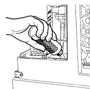
15. After the solution has circulated for 10 minutes push and release the Clean button. This starts the rinse process. Sanitize the ice storage bin while waiting. <P10.5>
