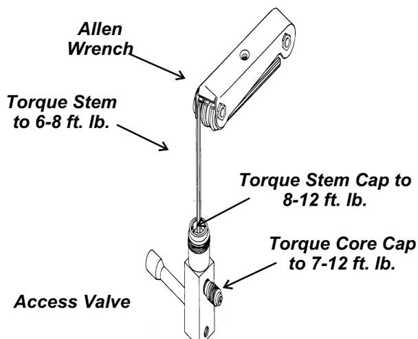
4. When service is complete, shut the discharge access valve first. Then, with the machine running and the middle hose outlet securely fastened to the manifold or refrigerant tank (closed) open both manifold valves. This allows any liquid refrigerant in the discharge hose to flow thru the manifold and into the suction side.
