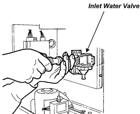
7. Unscrew the water valve from the water inlet tubing. Hold the barbed inlet fitting and rotate the valve.
