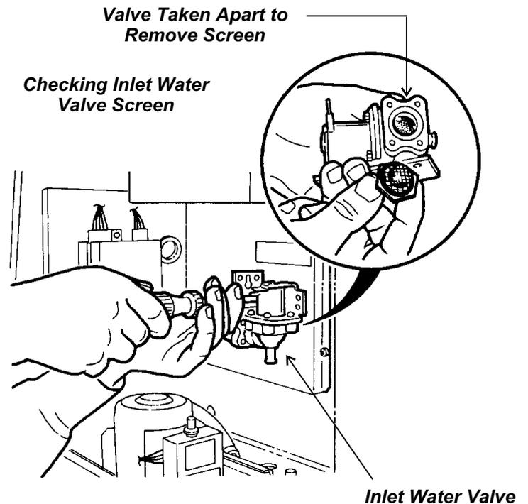
8. Examine the inlet screen, if dirty, brush off screen. Note: Screen is not replaceable, and may only be removed by taking off the covering bracket. The bracket forms part of the inlet water system, and must be water tight to the valve body, removal is not recommended.
