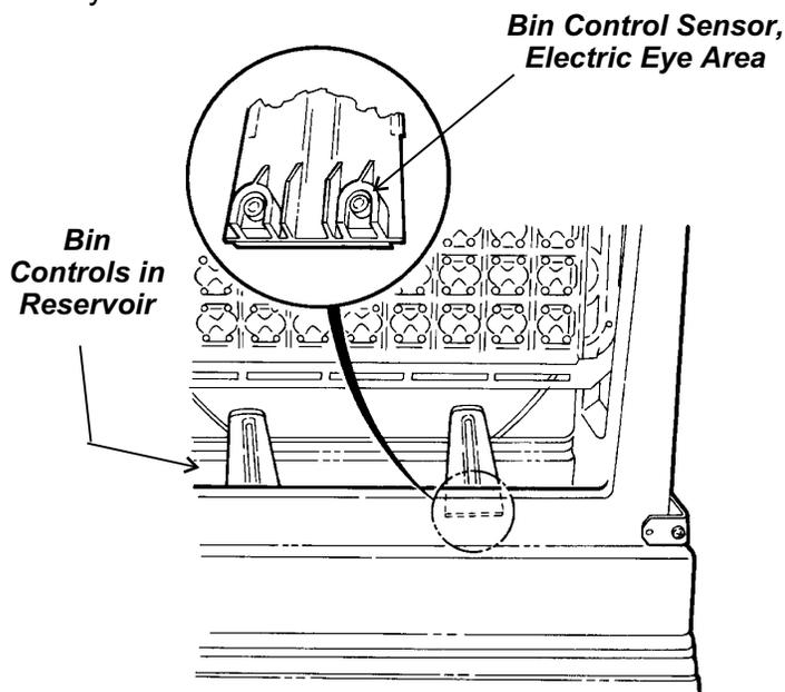
7. Examine the bottom of the brackets, there are two sensors in each bracket, check that they are clear of mineral build up. They may be wiped clean with ice machine cleaner to assist in removal of the build up.
