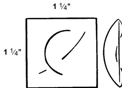
Note: Optimum performance will be achieved when the ice machine is adjusted to produce this size and shape of cube. The typical batch weight at this setting is between 8.25 and 9 pounds.
