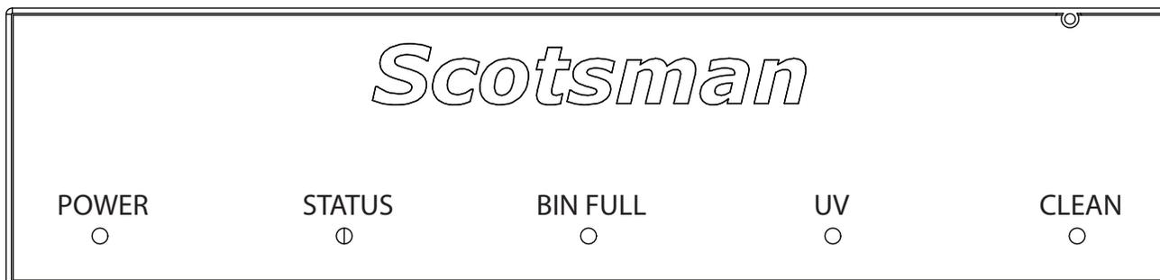
**Power:** When this light is ON, it indicates that there is power connected to the machine.
