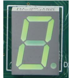
If a number code is triggered, the controller will stop ice making. A blinking code means it is a temporary condition. Example: A blinking *F* occurs during the ice making restart process; it stops blinking when the compressor starts.
