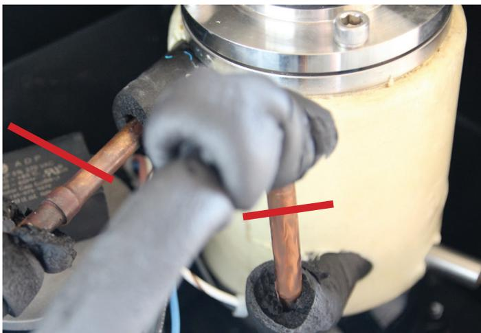
8. Cut evaporator inlet at the recommended spot.
