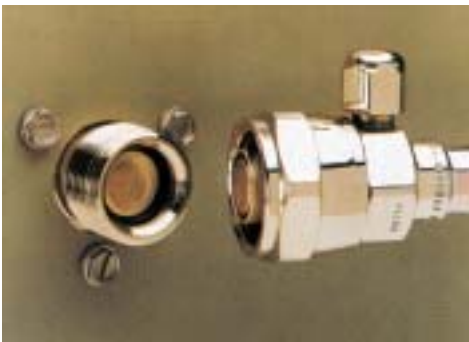
Clean and Lubricate Couplings
