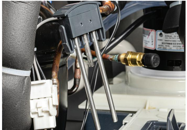
3. Wipe down probes with diluted scale remover to remove all traces of mineral build up. Rinse sensor probes with clean water (**do not submerge**) and then dry probes thoroughly.
