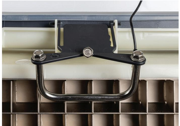
3. Wipe down the metal part of the sensor with diluted ice machine scale remover to remove all traces of mineral build up. Rinse sensor with clean water (**do not submerge**) and then dry thoroughly.
