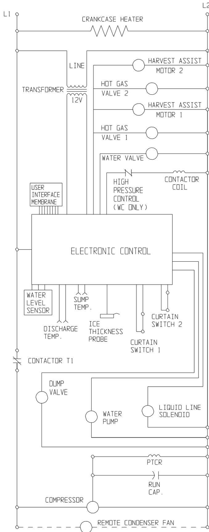
**Wiring Diagram, MC2648 Remote Single Phase**
