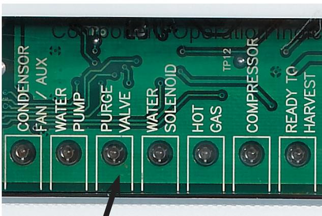
This light will be ON when the Purge Valve is powered.
