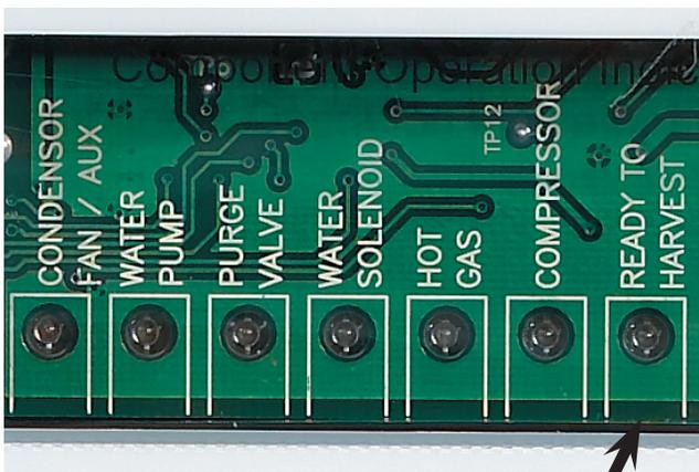
Ready To Harvest light is ON when water contacts ice thickness sensor.
