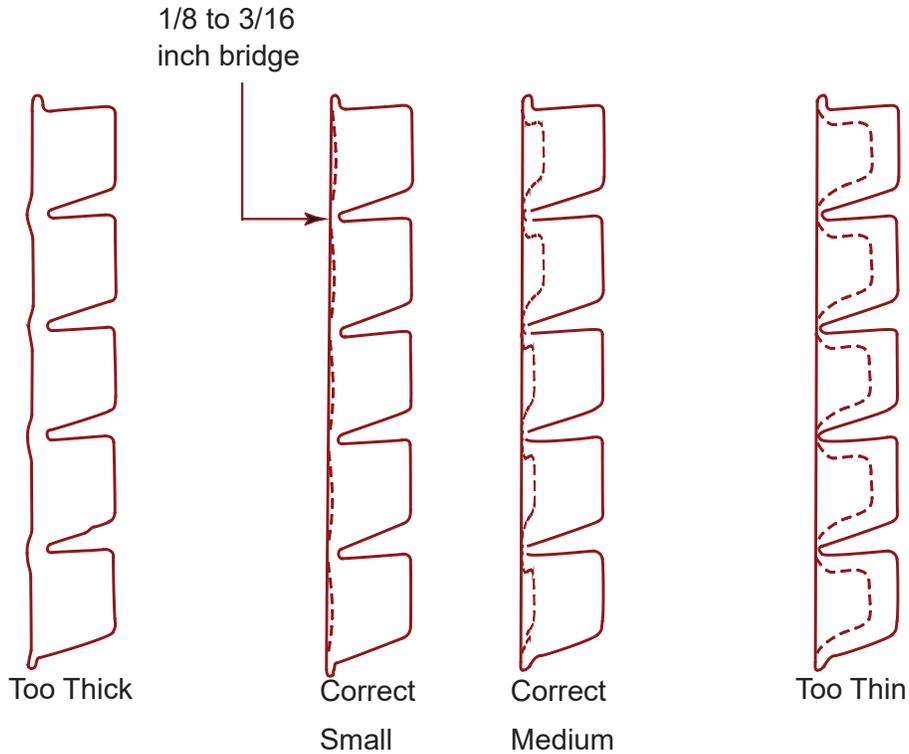
Caution: Do not make the bridge too thin or the machine will not harvest properly. Bridge thickness adjustments are not covered by warranty.
