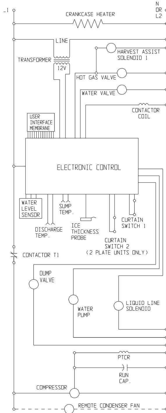
**Wiring Diagram MC0830 Air Three Phase**
