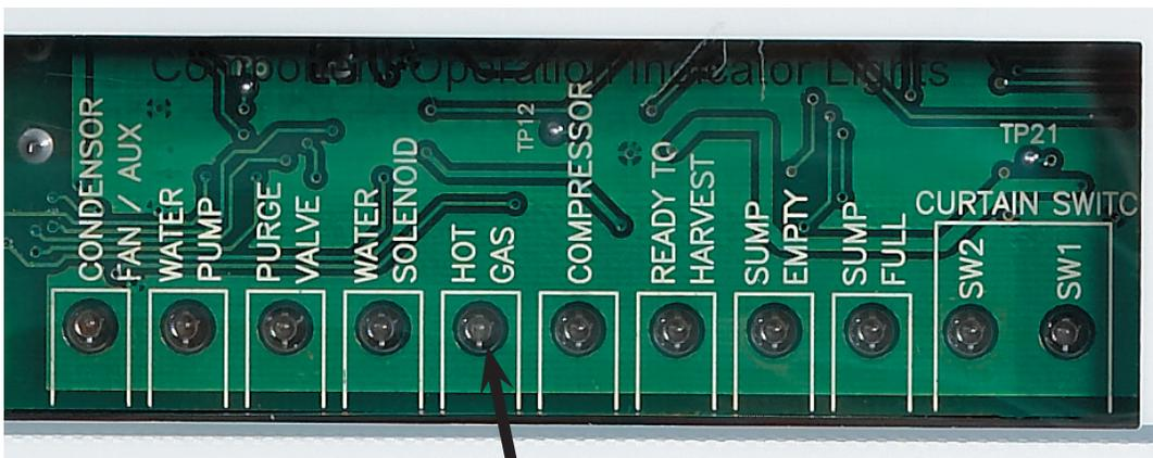
This light will be ON during harvest. Both the Hot Gas Valve coil and the Harvest Assist will have power when this light is ON.
