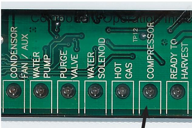
This light is ON when the compressor is operating.
