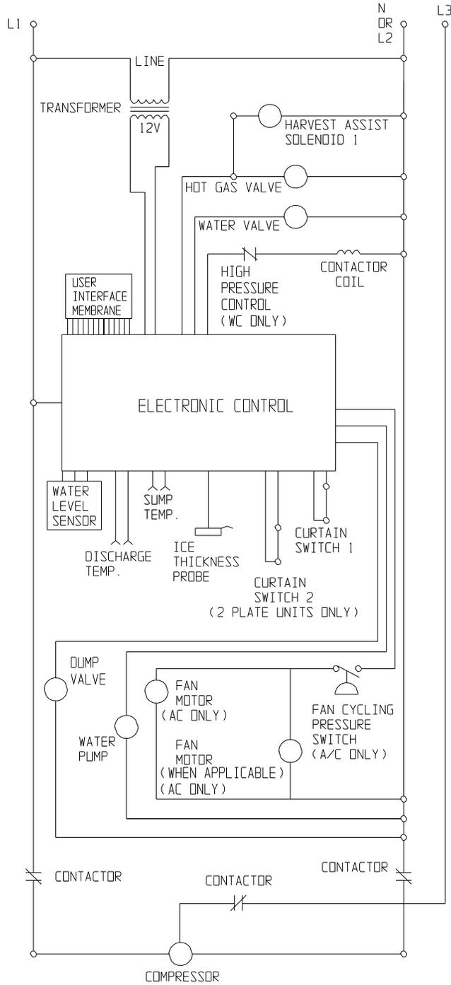
**Wiring Diagram MC1030 Remote Three Phase**
