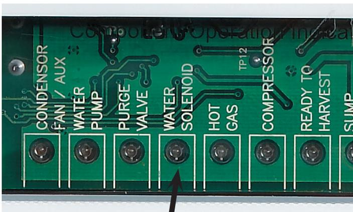
Light is ON when inlet water solenoid is in operation.
