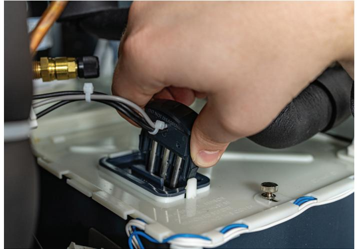
2. Press tabs to release sensor and remove.
