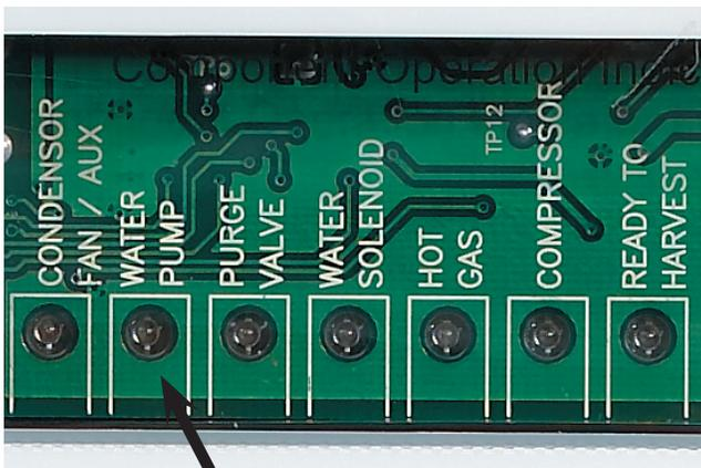
Water Pump light is ON when pump is operating.
