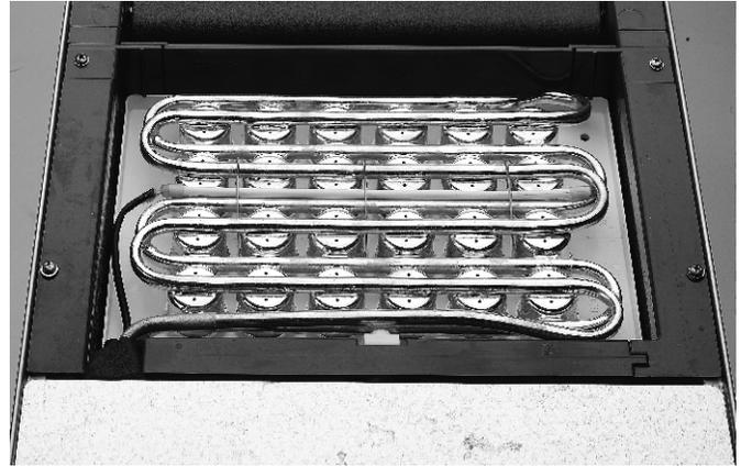
**Pour Scale Remover Over The Evaporator Section**
