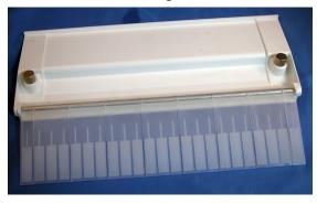
13. Locate elbows where water flows onto the evaporator platen.
