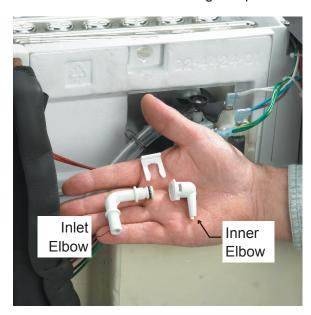
15. Pull water inlet elbow out of inner elbow.
