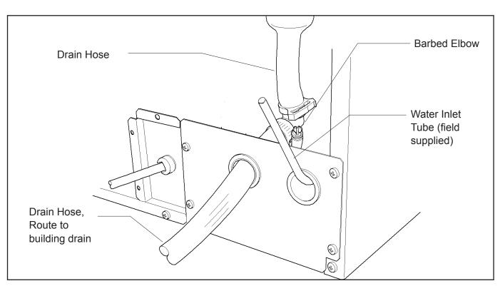
Back View, Gravity Drain Model
