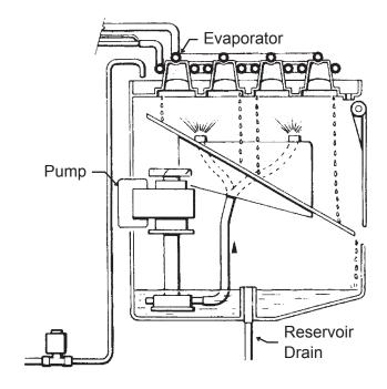
Freeze Cycle Water Schematic
