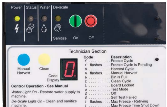
Controller Lights and Push Buttons
